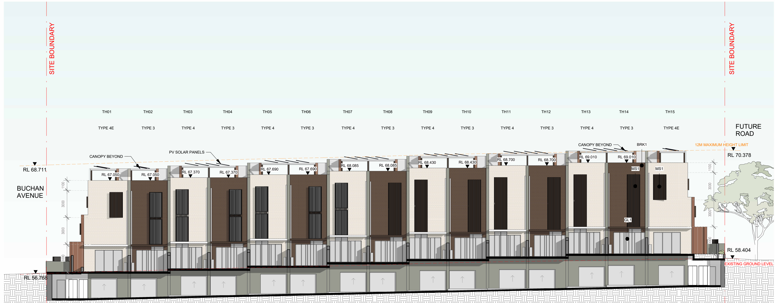
1 ELEVATION E (Section through Basement) SCALE 1 : 200
