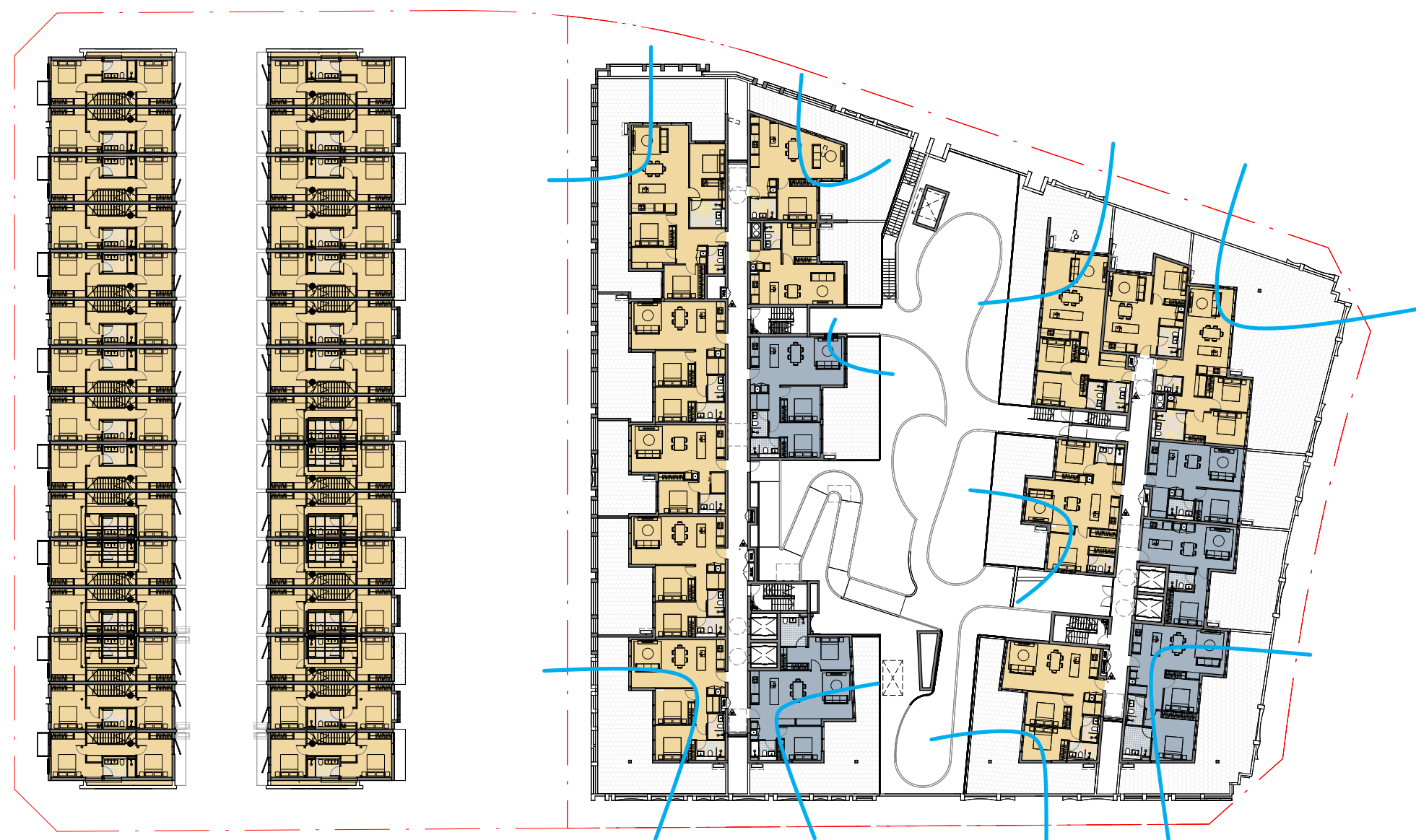
SOLAR & CROSS-VENTILATION - LEVEL 2
