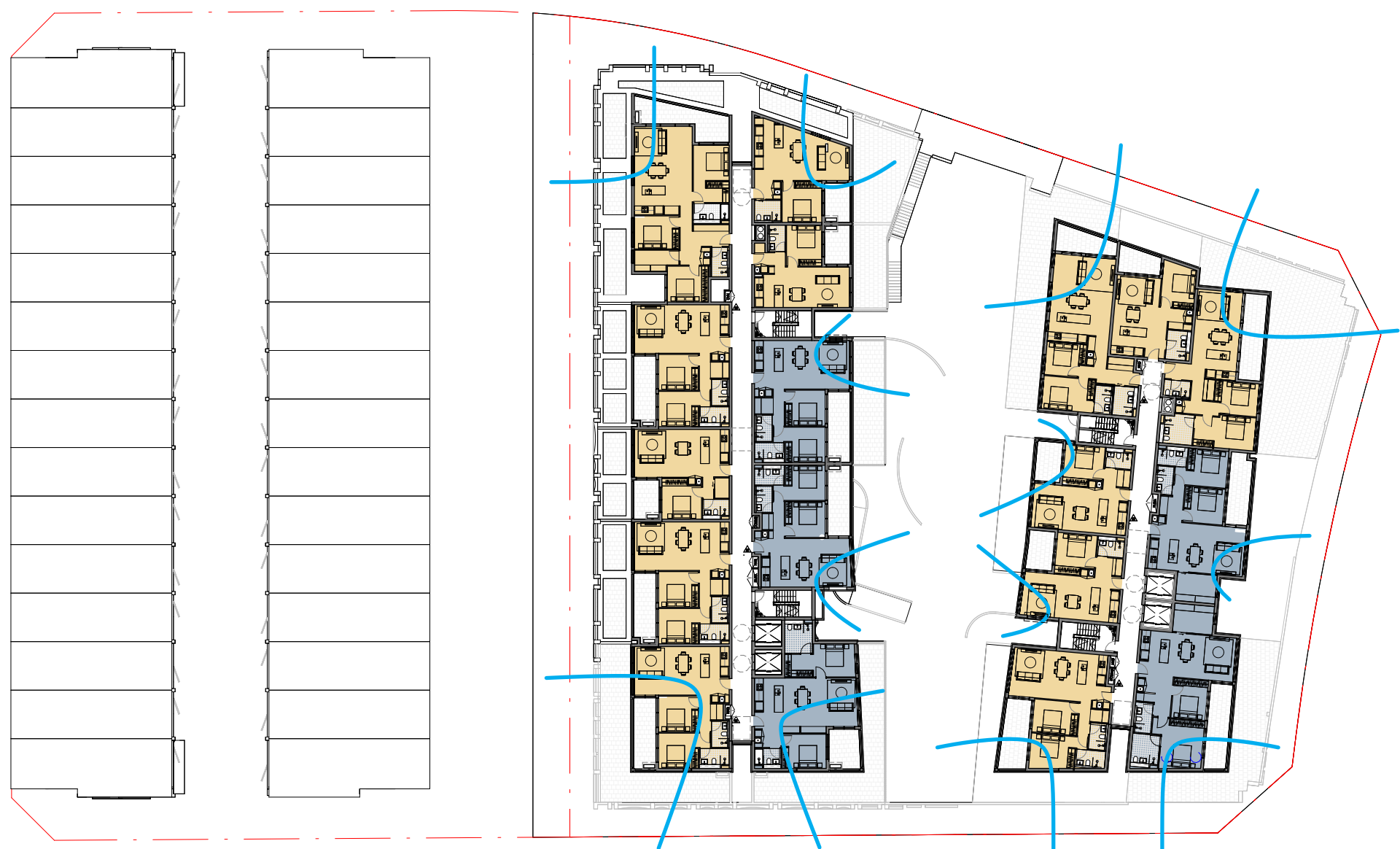
SOLAR & CROSS-VENTILATION - LEVEL 3
